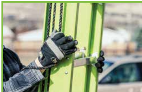
Side-mounted double-pulley reduces force required to raise the ladder and removes potential tripping hazard
